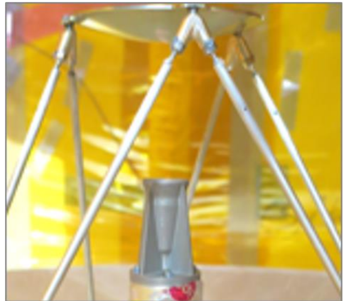
Fig. 7: Tri-band feed cluster manufactured using 3-D printing (after post-processing)
