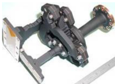
Figure. 9 K-Ka Band Dual CP Feed network
