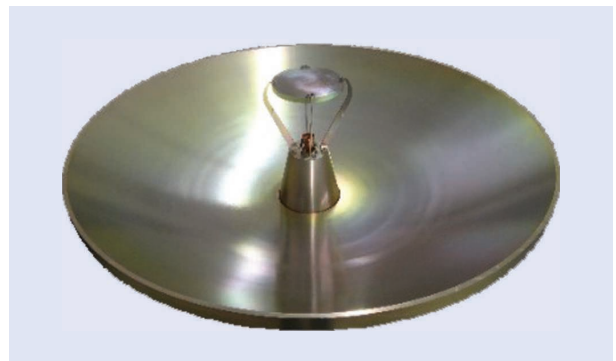
FIGURE 8. A Ka band antenna designed using the NewSpace approach.
