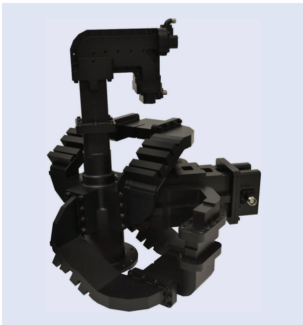
FIGURE 7. A space-qualified, dual-band dual-CP four-port C-band network using the NewSpace approach.
